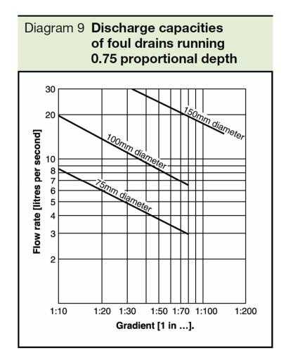
That implies that the maximum number of properties which should be connected to a 150  $\emptyset$  sewer is 100 [18  $\ell$ /s / 0.18  $\ell$ /s] provided that the load is only from foul water and not from a combination of surface water and foul.
